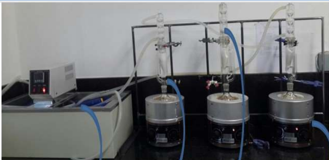
Cooling water for circulation in condenser
