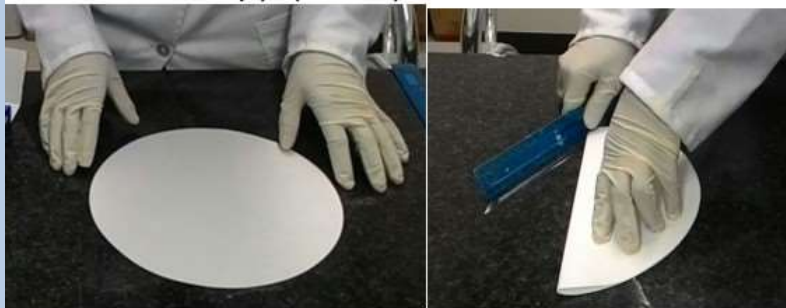
Fig 2; Making a thimble from a filter paper
